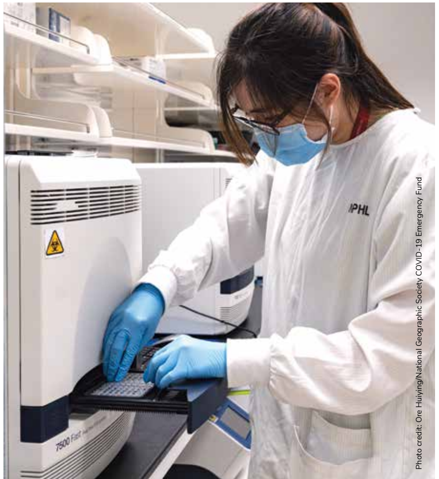
Medical technologist loading sample strips into a real-time PCR system for detection of pathogen
