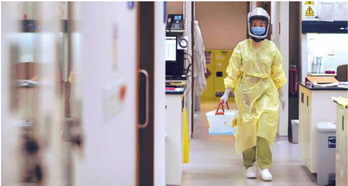
Transporting infectious substances such as SARS-CoV-2 specimens safely in a leak-proof container within the laboratory
